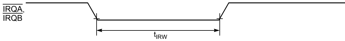
Figure 10-6 External Interrupt Timing (Negative Edge-Sensitive)
