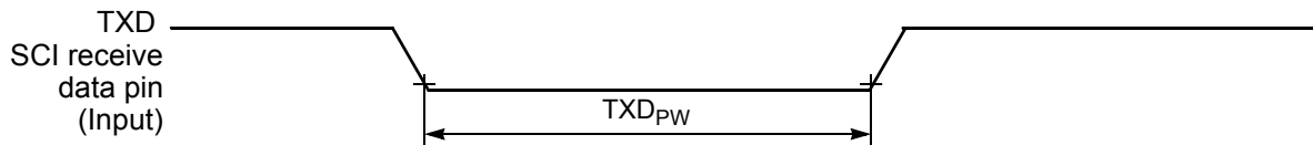
Figure 10-17 TXD Pulse Width
