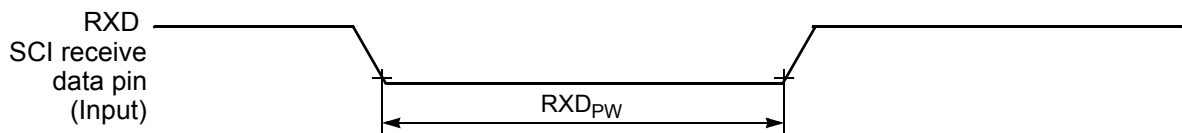
Figure 10-16 RXD Pulse Width
